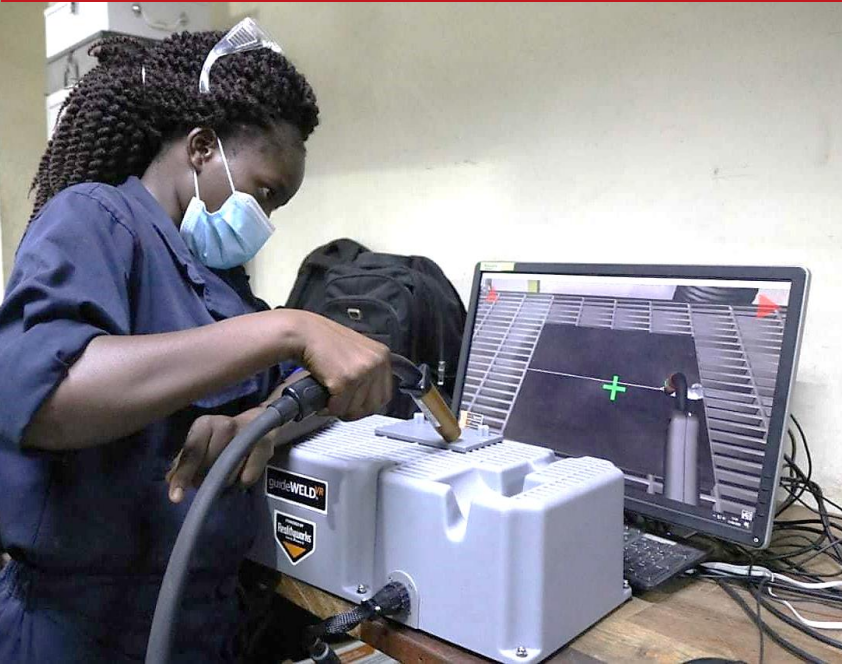
Welding simulator using Augmented Reality
