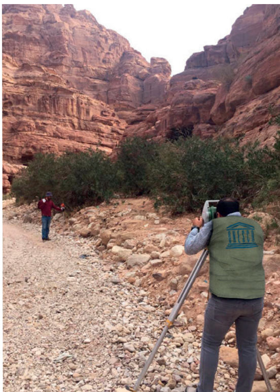
▲ TOPOGRAPHIC SURVEY OF THE CHANNEL WADI AS-SIYYAGH © UNESCO
