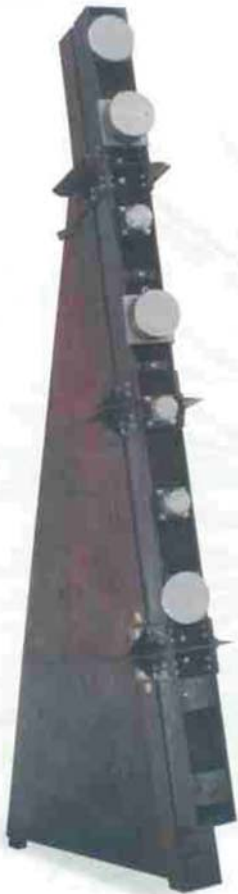
Instrumented steel wedge to measure avalanches
