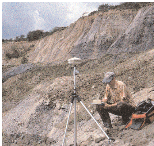
Surveyor in Black Ven carrying out measurements using a satellite positioning system. There are extensive datasets on many of the landslides, which enable the sometimes rapid changes in form to be tracked over many years.
