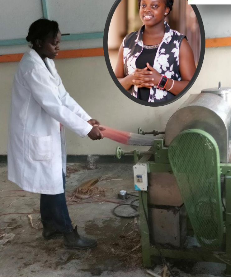
Decorticating process with machine fabricated at KIRDI
